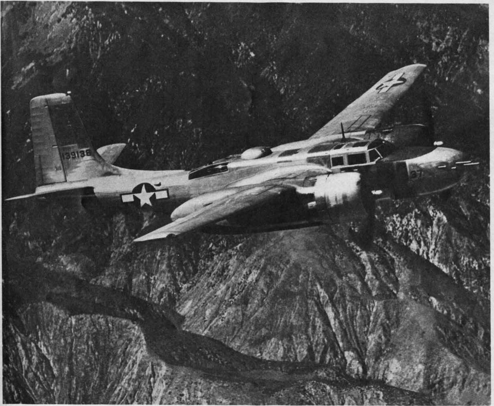
Huge square tail dominates the A-26's appearance in most views, and is its chief identifying characteristic. The airplane's Pratt & Whit-
